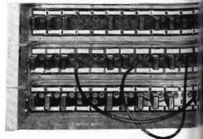
Video Jack Panel, MI-26245. For patching and/or sync signals. Includes 12 groups of contact assemblies (3 per group). Video jack plugs and cords.
