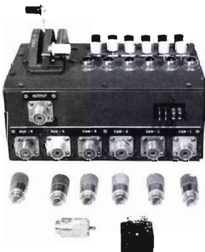
Rear view of Field Switching Control showing coax connectors and Jones plug supplied
