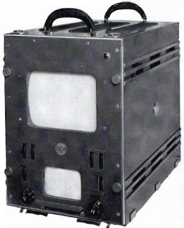
TM-5A Master Monitor shown mounted in Field Carrying Case, MI-26521
