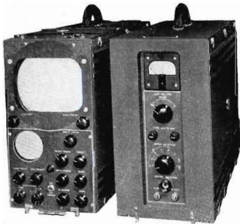
Field Camera Control Unit and Field Power Supply
