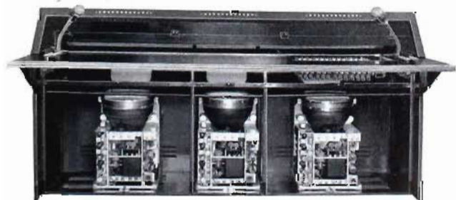
Program Monitors, TM-1A, shown installed in Program Director's Console
