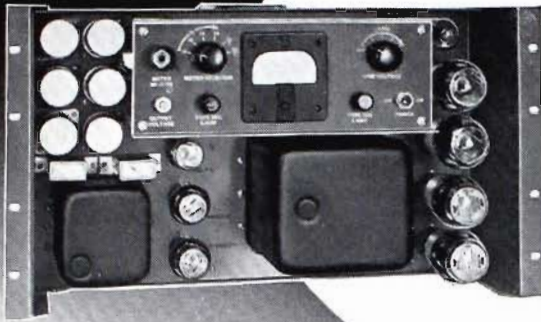
Regulated Power Supply, TY-25A. Provides well-regulated d-c source at loads from 200 to 300 ma. Output is adjustable between 260 and 290 volts. Less than 0.5% variation between minimum and maximum load.
