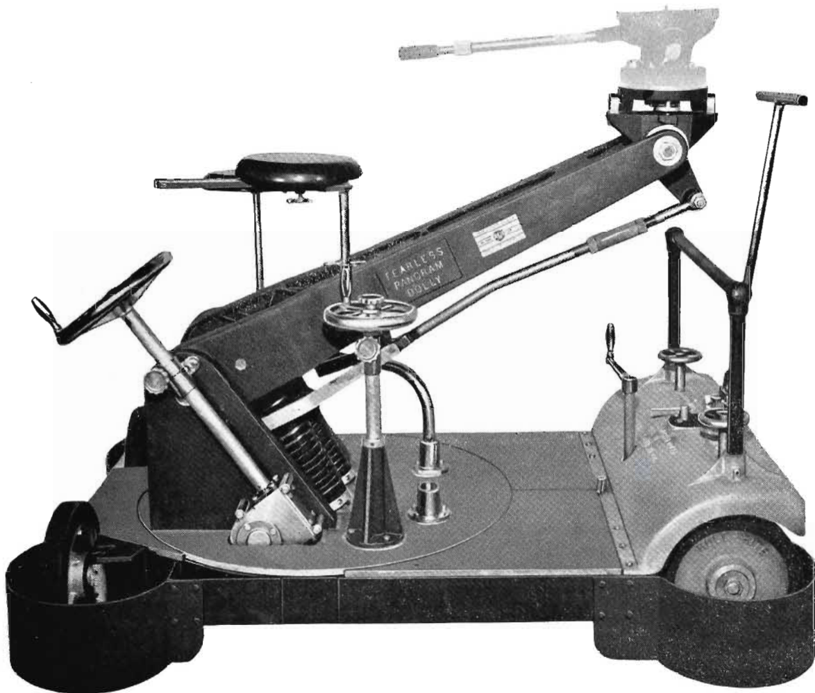
View showing rear wheels turned at right angles. Friction head for mounting camera is supplied separately as MI-26205.
